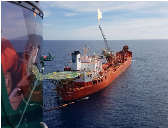
Offloading of Oil to a Shuttle Tanker from the “FPSO Intrepid Balanghai”
